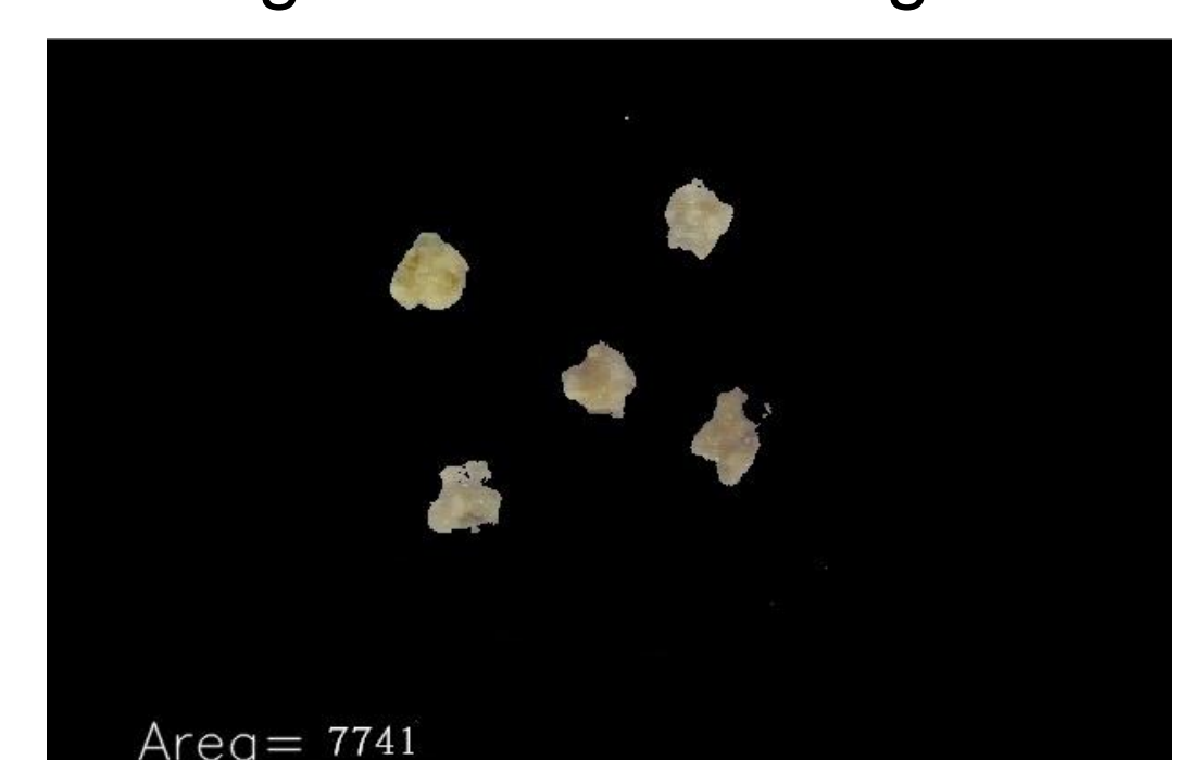
3. The image after thresholding and the area in pixels
